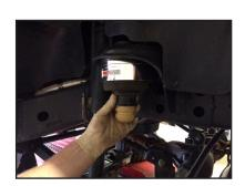
**STEP 12:** Reinstall OE coil springs into their original position.
