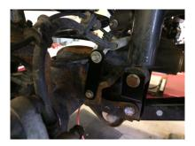
**STEP 16:** Install caster/pinion angle cam bolts, included with this kit. Wheel alignment will be required after installation is complete.
