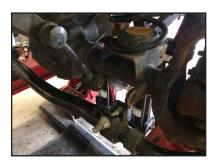
**STEP 6:** Install coil spring clamps, if available. This will simplify removal & rein-stallation of coil springs.
