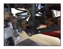
STEP 8: CAREFULLY lower front axle, then remove OE coil spring, and OE upper rubber insulator. RETAIN OE INSULATOR FOR REINSTALLATION IN STEP 11.
