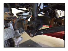
**STEP 5:** Disconnect one end of each front sway bar link.
