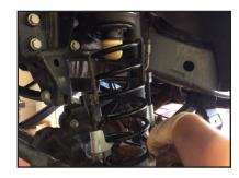
**STEP 9:** Determine your desired front lift height from 1.5" to 3.0", combining spacers as required. The largest spacer w/ logo should always be the **LOW-EST** spacer installed. The actual lift value will be the same as the thickness of the combined spacers.
