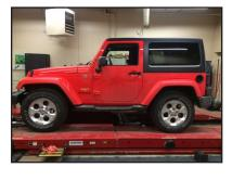
**STEP 2:** Position vehicle on a stable, flat surface or automotive lift. Suspend front wheels, lift-
