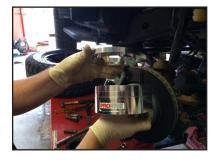
**STEP 10:** Install spacers over front bump stop, largest spacer at bottom, and secure to the coil spring pocket with included bolt & nut hardware.
