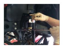
**STEP 11:** Reinstall OE rubber insulator, removed in Step 8, as shown.
