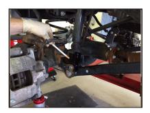
**STEP 15:** Install brake line relocator brackets on each side of vehicle using included hardware, as shown.
