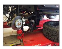
**STEP 4:** Unclip lower ABS, vacuum & brake line brackets to allow slack.
