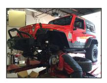
**STEP 3:** Support lower control arm & spindle assemblies, then remove front wheels.
